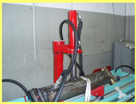
Cylinder locking system with pushing Hydraulic cylinder. ACSTT0000029
