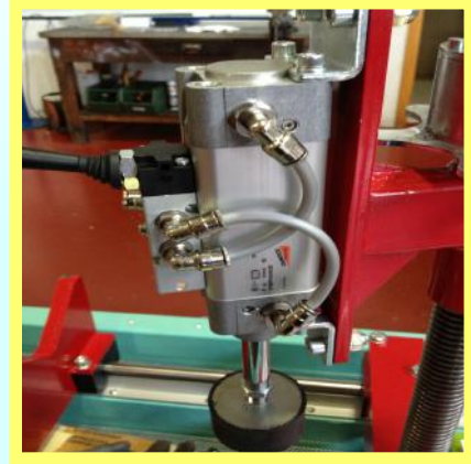
Cylinder locking system with pulling hydraulic cylinder. ACSTT0000030
